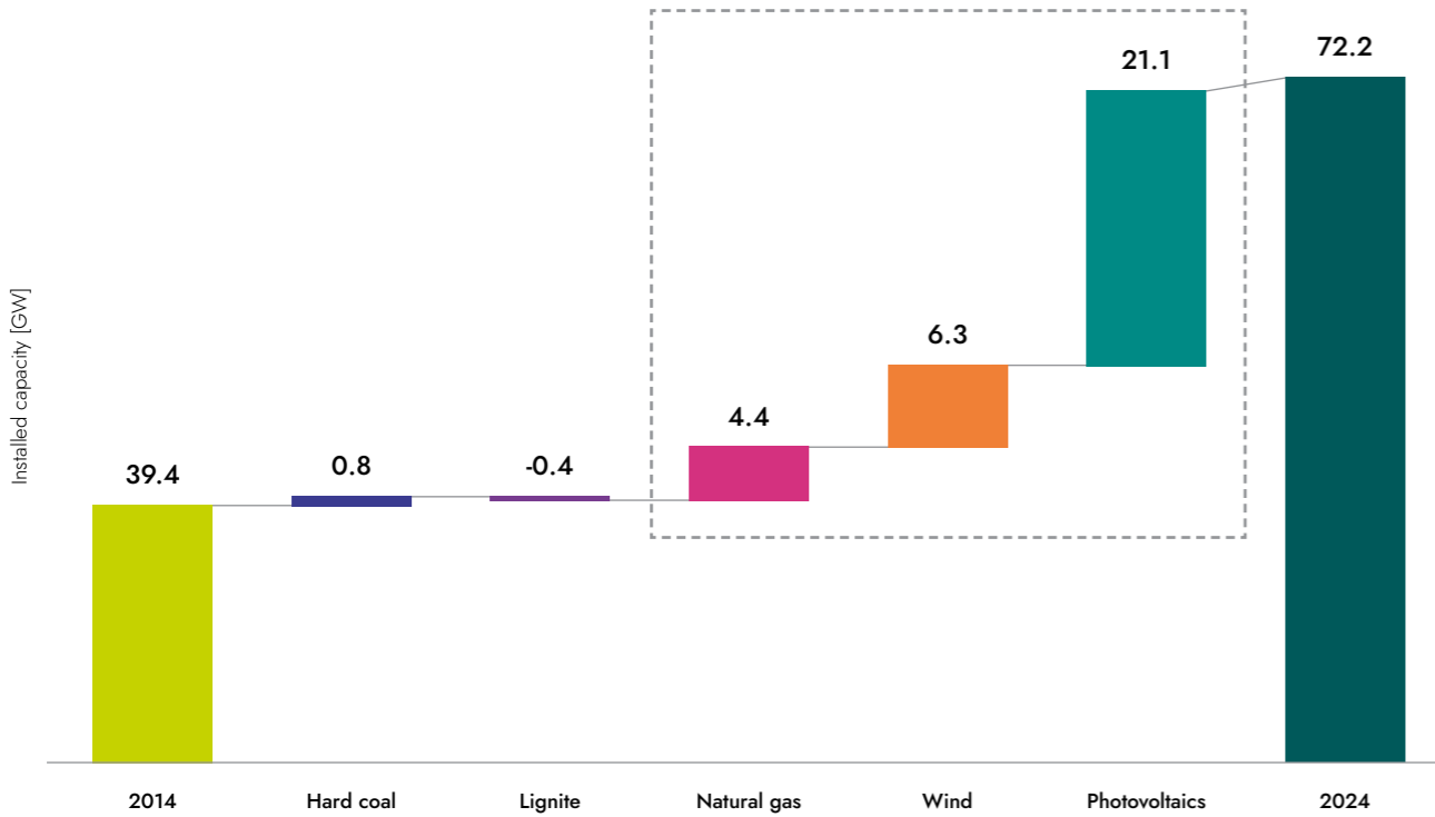
Fig. 3. Increase in installed capacity of renewable sources and flexible, controllable sources in Poland from 2014 to 2024
